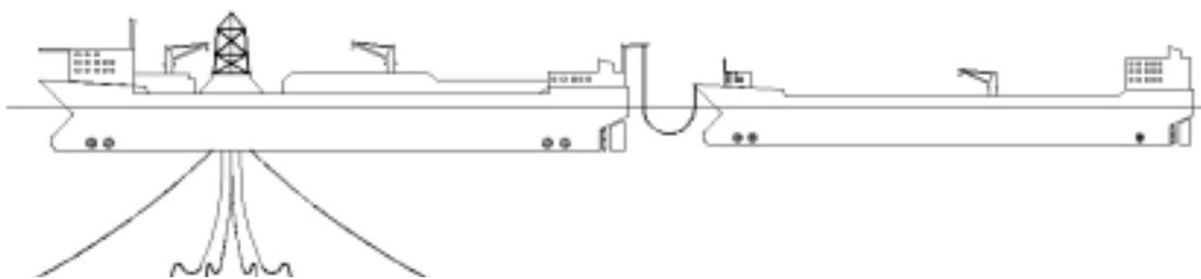
**Figure 5. FPSO Offloading to a Shuttle Tanker**
