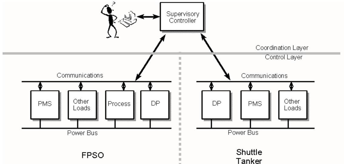
**Figure 4. Coordinated Control for Two Vessel System**
