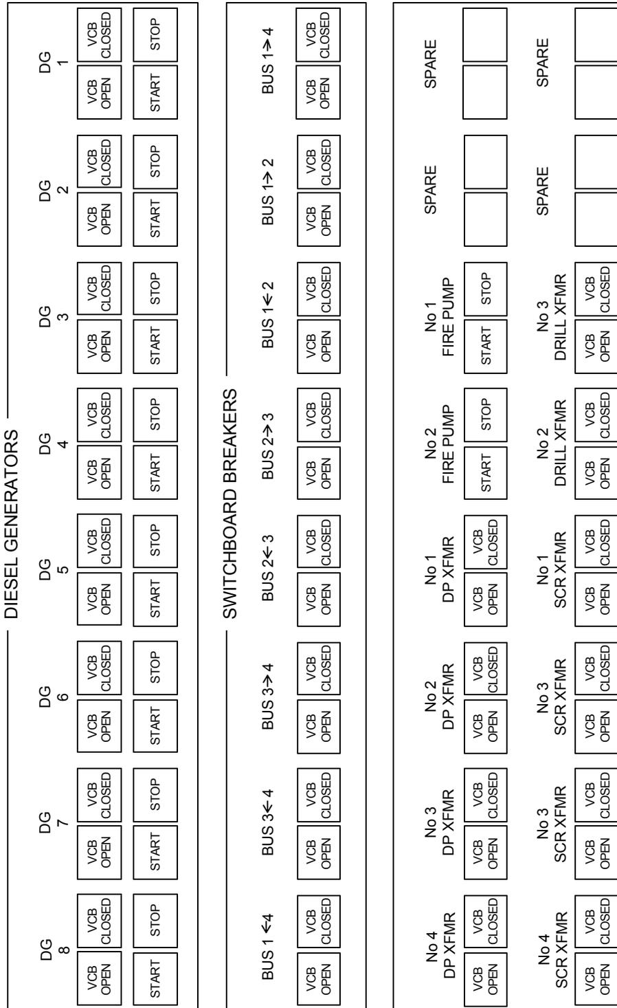
**Figure 4** Layout of the Initial Power Management Control/Display Panel for “Ocean Confidence” DP System
