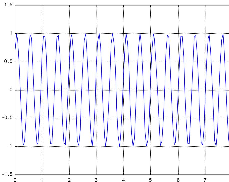
Figure 1 shows a sinusoidal pulse with a frequency of 19.8 kHz with a duration of 800  $\mu$ s. This is a typical waveform for NAUTRONIX RS5D SBL systems.
