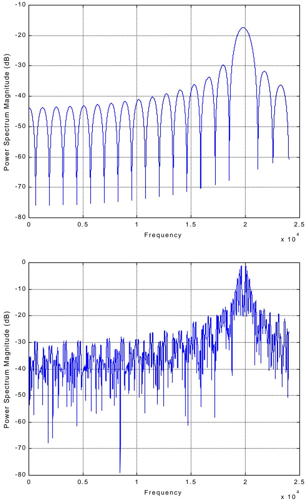
Figure 3: Power Spectrum Density of a 800 us Pulse and 10 ms PSK Pulse
