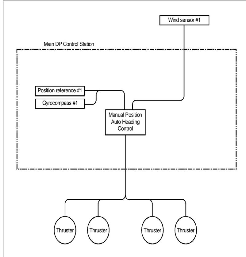
would be operations where the positioning function is not considered to endanger human lives, or cause major damage in case of failure. An example of a DPS-0 system is shown in Figure DPS0.
